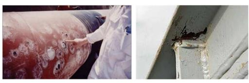
Typical example of detrimental effects of soluble salts under a coating system (surface corrosion). Osmotic blistering (*left*); loss of adhesion due to underfilm corrosion (*right*).
